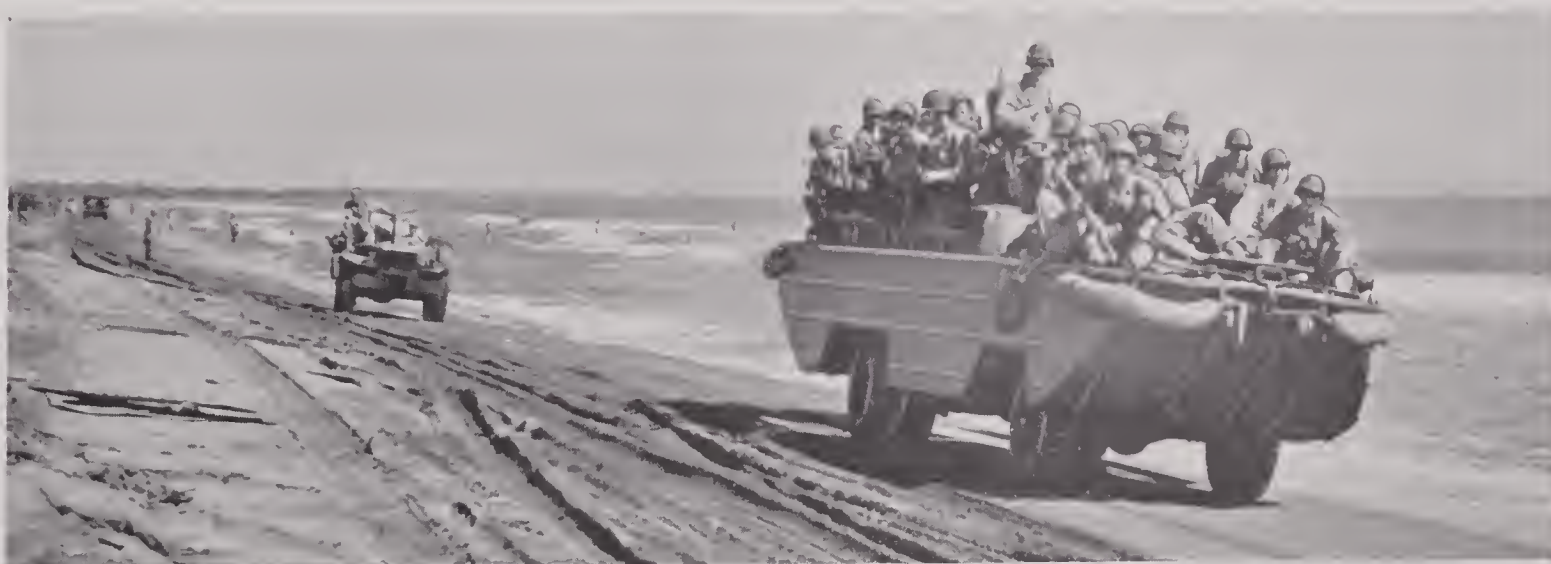
FIGURE 36. DUKW transporting troops on north coast of New Guinea. Hard sand beaches along this coast served as temporary roads.
